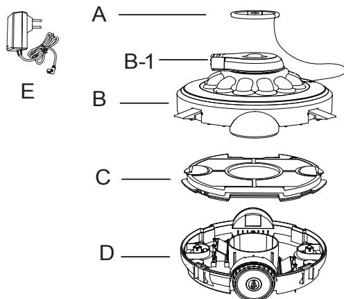
There is a rotation jet head at the upper cover, the water is passing from bottom to the jet head to make the robot moving. While facing obstacle, the jet head turns around 180 degrees, the robot rounds the obstacle and moving by another line. The rubbish is collected and installed by the bottom filter cabine.
