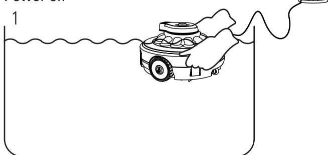
Turn on the switch, loosen the rope on the float, put the robot horizontally into the pool, and wait for the robot to sink freely to the bottom. (if the product is not put into the water, the machine will not rotate because the machine has the function of "stop when leaving water").
